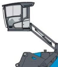
Cab system vertically adjustable and horizontally adjustable
